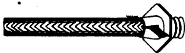
Fig 4 Terminal pinched to- gether, by means of Gas Pliers to firmly grip the insulation.
