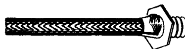
Fig 5 Wires bent close to Ter- minal (on one side) ready for soldering.
